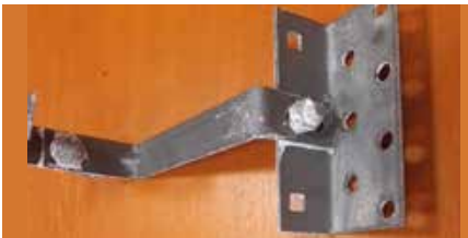
Photo 3. Photo after 320 h magnelis including bolt in hot-dip galvanized coating.
