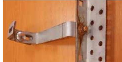
Photo 4. Photo after 320 h sample of acid resistant steel 1.4301 with A2 stainless steel bolt
