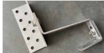
Photo 2. Photo before inserting sample of acid resistant steel 1.4301 with A2 stainless steel screw into the salt chamber.
