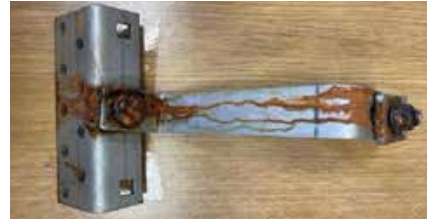
Photo 6. Photo after a full 720 h cycle sample of 1.4301 acid-resistant steel including A2 stainless steel screw.
