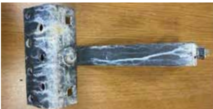
Photo 5. Photo after a full 720 h magnelis cycle including the bolt in hot-dip galvanized coating.
