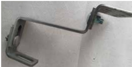
Photo 1. Photo before inserting the Magnelis® sample including the bolt in hot-dip galvanized coating into the salt chamber.
